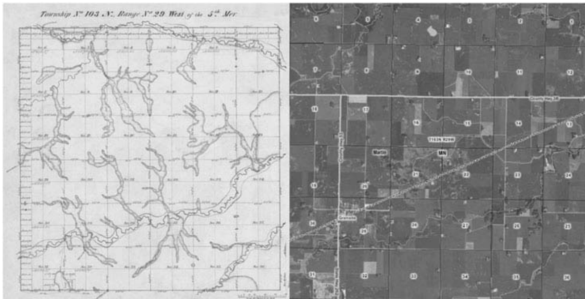
Figure 3. General Land Office survey map of 1855 showing small tributaries to Elm and Center Creeks, Minnesota. Many first-order and second-order streams that were wide (100–400 m) and highly sinuous (referred to as 'sloughs' in survey notes) have been graded into farmland, channelized and/or drained by subsurface pipes. Some surface ditches were constructed in areas where streams did not previously exist. Overall there was a net loss in headwater stream length of approximately 20%. This figure is available in colour online at wileyonlinelibrary.com/journal/rra .
