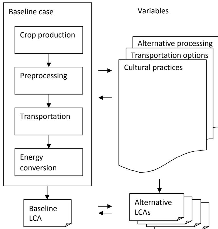
**Figure XX. Parametric LCA framework for evaluation of alternative practices in biomass-based energy production system**
